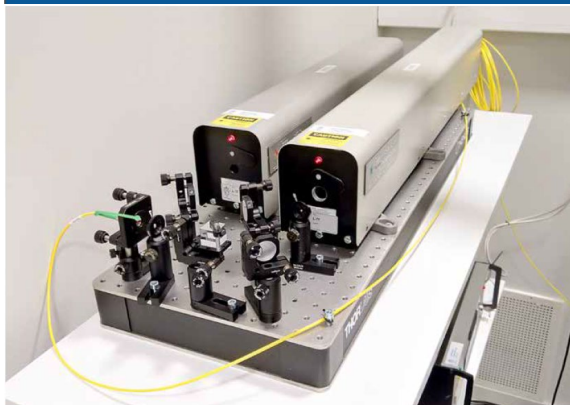
Figure 2. Optics for SM fibre coupling for lasers of an upgraded GBI.
