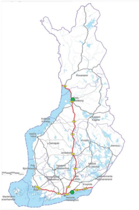
Figure 5. The core network and comprehensive traffic network in Finland 9 . Numbered circles indicate potential locations for the HRSs. Filled green dots illustrate the possible locations for semi-centralised hydrogen production facilities in Porvoo and Oulu 9 .
